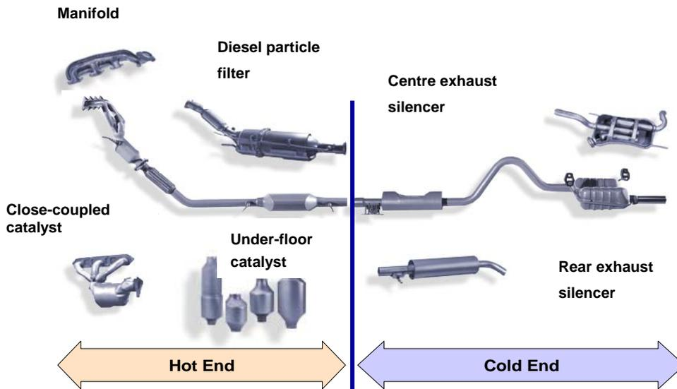
Hot end and cold end of an exhaust system
